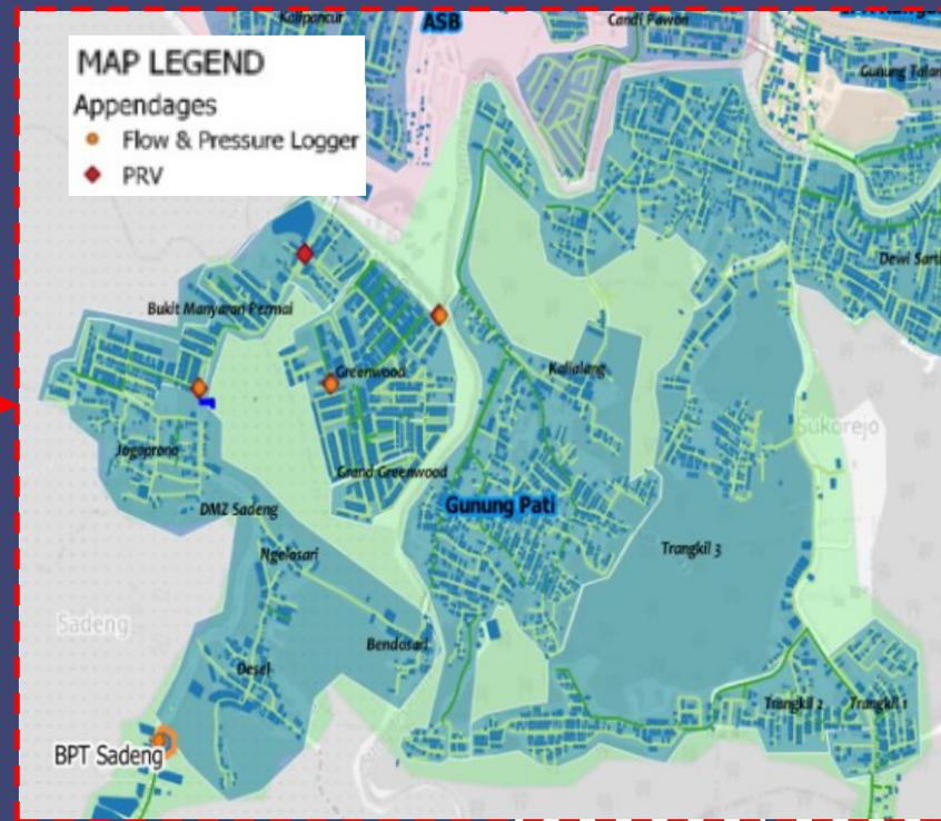
The 'Gunungpati' Supply Zone (7,500 connections, 13 DMAs) showing the location of a selection of the 13 installed flow/pressure (data) loggers; measurement results of which were used to guide Active Leak Detection Activities and Physical Loss reduction interventions (see overleaf): pipe repair, PRV installation (pressure management), pipe replacement
